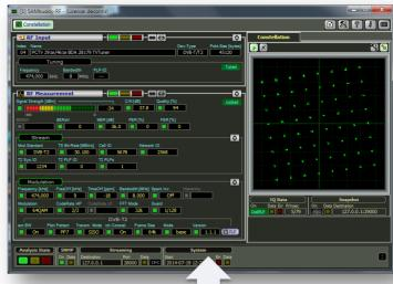
All relevant RF measurements including the constellation as well as important stream- and modulation parameters are also visible at one glance during the entire test drive.
